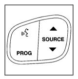
(w<sup>2</sup>/<sub>€</sub> : If your vehicle is equipped with the steering wheel control buttons you can use them to interact with the OnStar<sup>®</sup> system.
